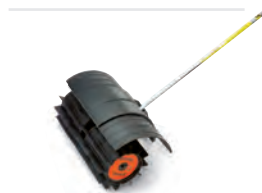
KW-KM STIHL PowerSweep™ ATTACHMENT Heavy-duty rubber flaps clean up caked dirt on concrete, move pebbles and sand from turf and water and light snow from hard, flat surfaces.
