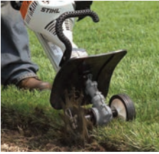
FC-MM BED EDGER ATTACHMENT Cut defined edges and separate the grass from the planting area.
